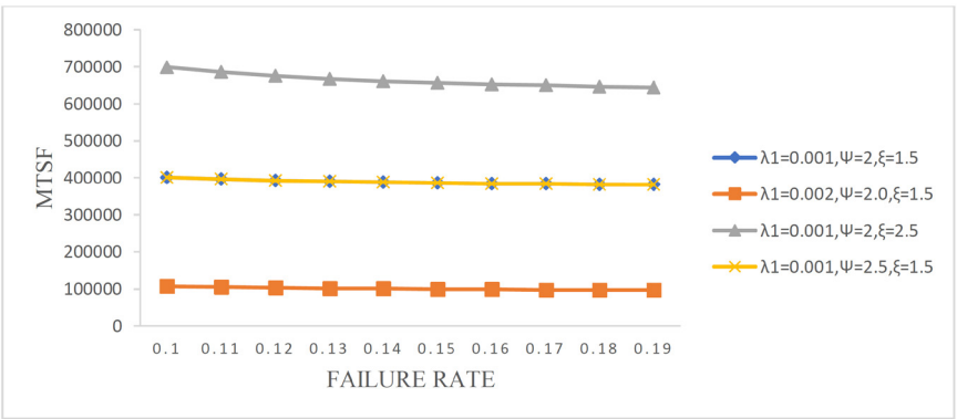
Figure 2 MTSF Vs Failure rate of phase-I unit
