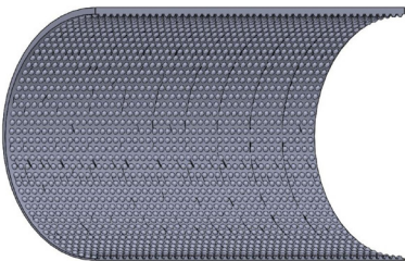
Figure 20 Hemispherical Dimple Texturing Pattern
