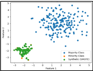
Figure 3 SMOTE-based sampling visualization showing majority samples, original minority samples, and synthetic minority instances generated through interpolation in the feature space.
