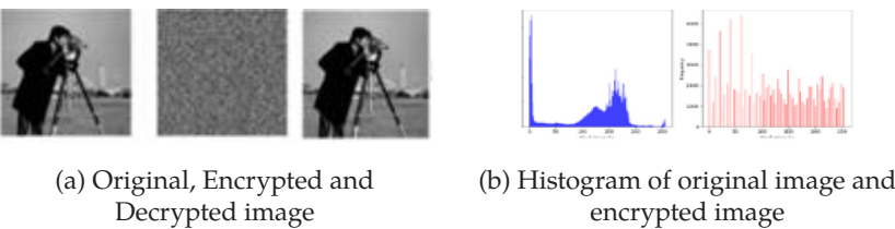
Figure 2 Original and encrypted image generated from the proposed work and their Histogram analysis
