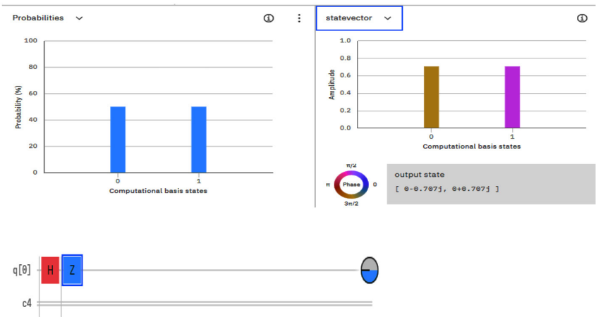
Figure 13 Superposition state 's Qubit with Z Gate
