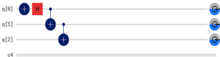
Figure 15 Entanglement of three qubit (GHZ State)
