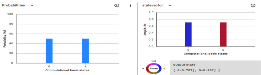
Figure 14 Superposition state 's Qubit with Z Gate
